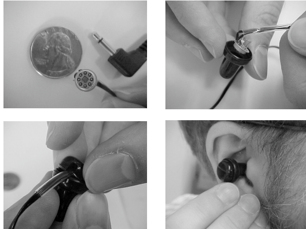
Figure 1.9: Photographs of earphone construction.
