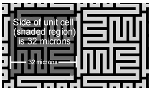
Fig. 2. The layout of the serpentine mesh pattern that defines the membrane. Beams are represented by gray, gaps by black. One unit cell is 32 \mu\text{m} across.
