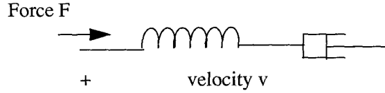
Fig 2.6 A branch with series connected spring and damper elements
