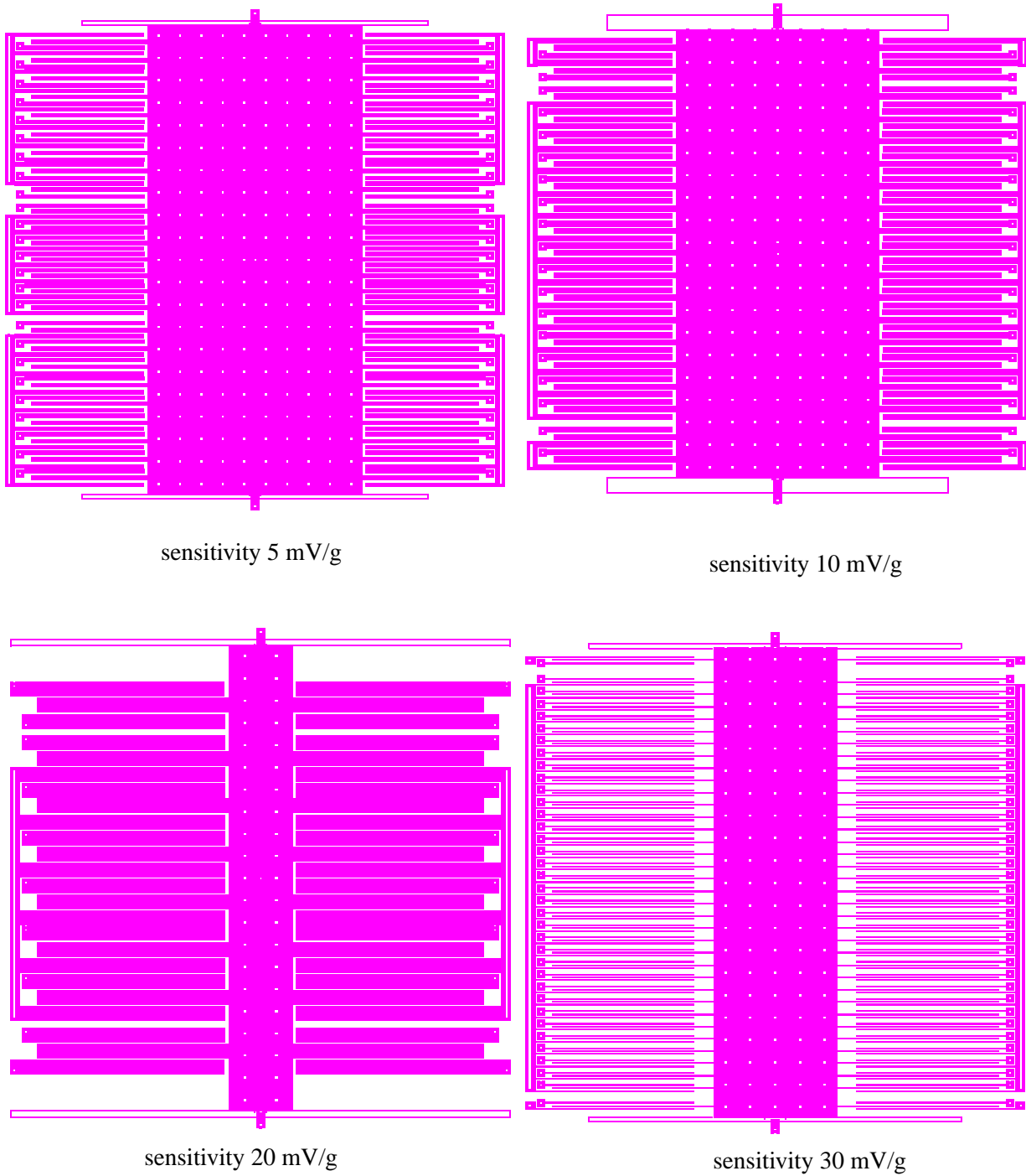
Figure 16(b). Synthesized accelerometer layouts for minimize-noise with 4 sensitivity specs in closed-loop operation.
