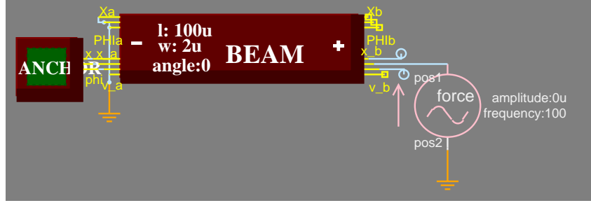
Figure 18. Schematic representation of 100 \mu\text{m} long by 2 \mu\text{m} wide cantilever beam with AC force source actuating it in the y-direction.
