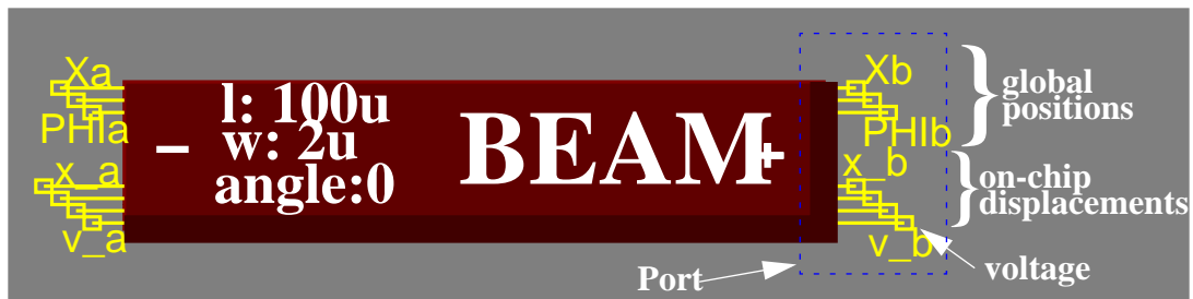
Figure 31. Beam Symbol, with ports, global position nodes, chip displacement nodes, and electrical nodes.
