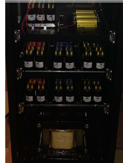
R-L-C Load Circuit
