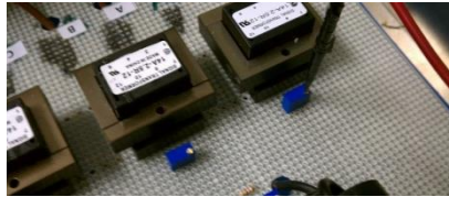
PTs and Calibration potentiometer
