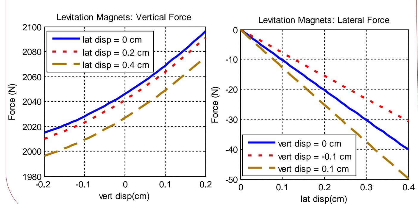
Force plots for the total magnetic bearing system, including both the levitation magnets and the Halbach array stabilizer
