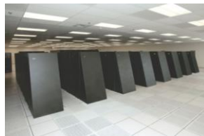
BlueGene/L 65,536 dual-core CPUs 16 TB RAM, 360 Tflop/s 0.045 byte/flop
