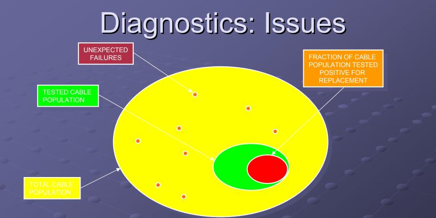
If number of replaced segments is smaller than failure forecast, unexpected failures will likely occur Even if the number of replaced segments is equal to the failure forecast, there may (and probably will) be unexpected failures in the untested population 25
