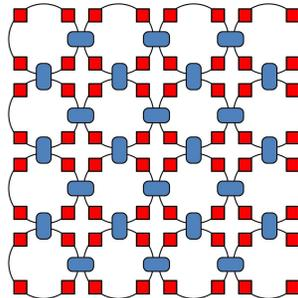
Figure 6: mesh of rings topology
