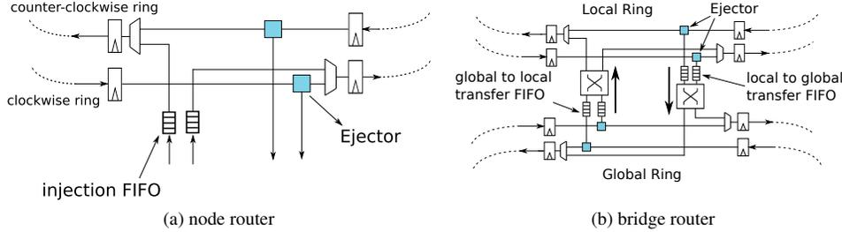
Figure 7: High-level block diagrams of (a) a node router and (b) a bridge router
