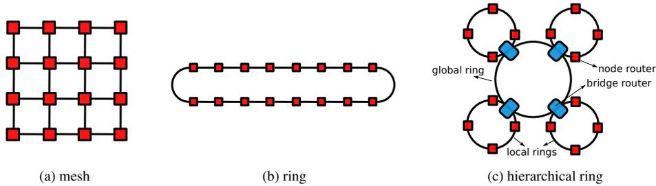
Figure 3: Topology for (a) mesh, (b) ring, and (c) hierarchical ring networks.
