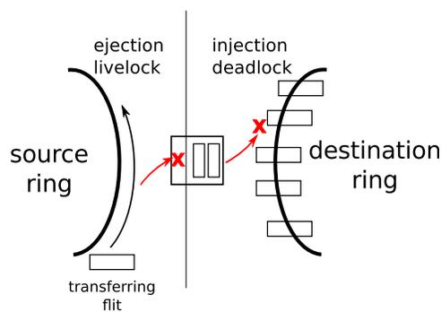
Figure 8: Ejection livelock and injection deadlock in a multi-ring system.
