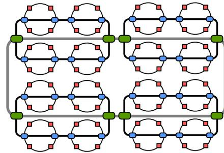
Figure 5: Three-level hierarchy for an 8x8 network.
