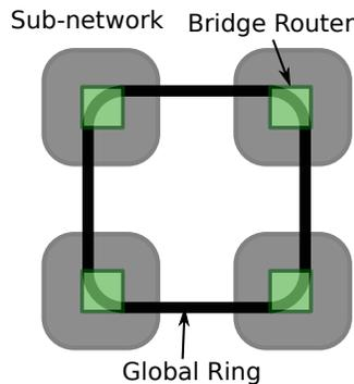
Figure 12: Hierarchical ring topology scaled to 64 cores
