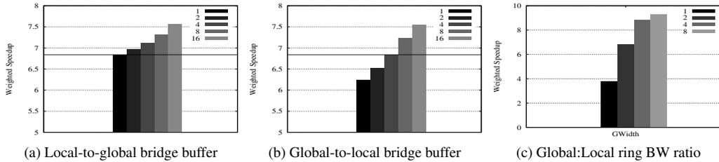
Figure 16: Performance sensitivity to buffer sizes and the global ring bandwidth in a 4x4 network.
