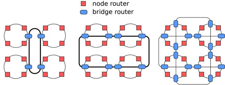
Figure 4: 4-bridge, 8-bridge and 16-bridge Hierarchical Ring topology
