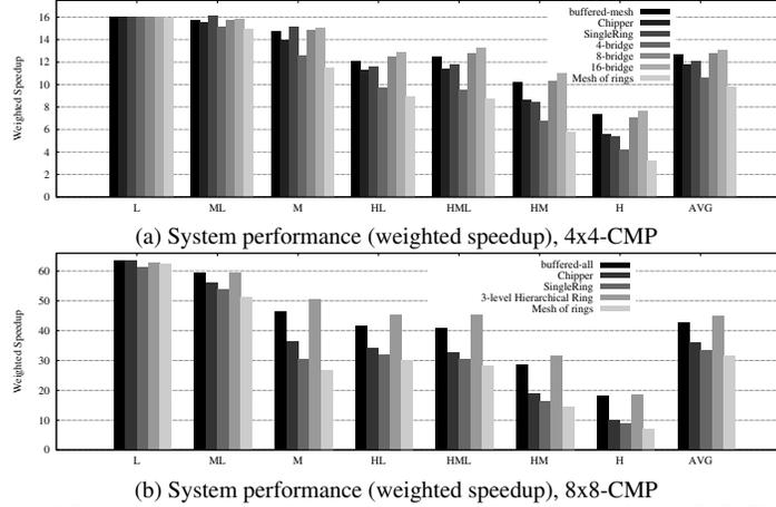
Figure 13: Application performance comparison for 4x4 and 8x8 CMPs.
