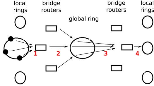
Figure 9: End-to-end delivery guarantee: (1) the ejection guarantee ensures that flits injected from nodes on a local ring are ejected for transfer at the bridge to the global ring. (2) The injection guarantee ensures that flits in the bridge router’s FIFO are injected into the global ring. Similarly, the ejection guarantee (3) and injection guarantee (4) ensure traffic moves from the global ring to its destination local ring. The Dual-Transfer Swap rule breaks any circular dependencies.
