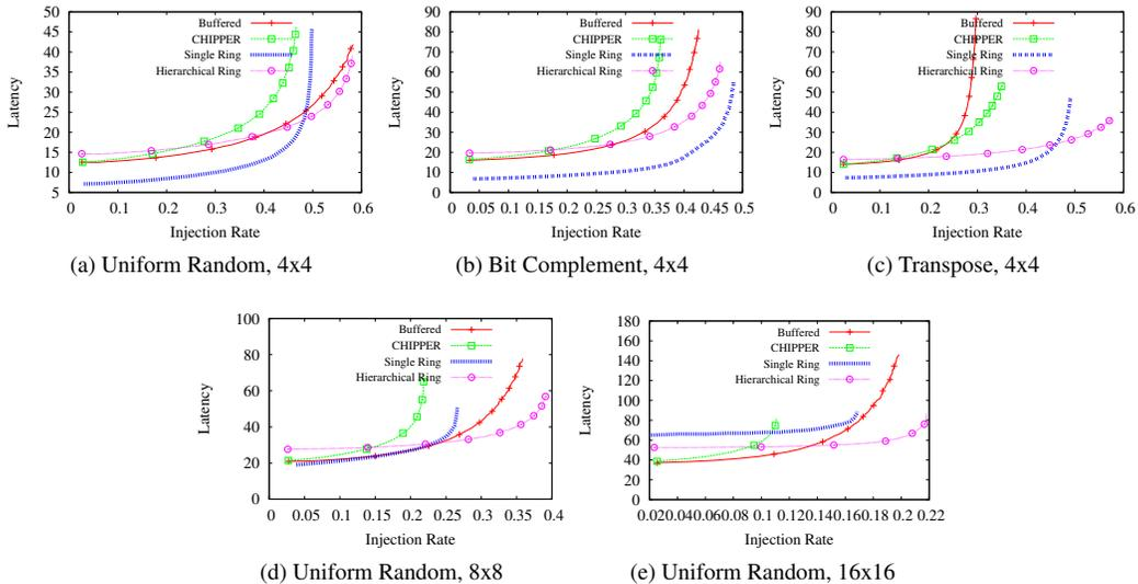
Figure 15: Synthetic-traffic evaluations for 4x4, 8x8 and 16x16 networks.
