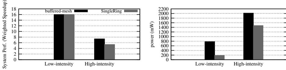
Figure 1: Performance and average network power for 16 nodes, in mesh and ring interconnects.
