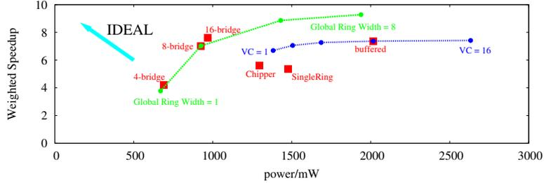
Figure 17: Performance and power in a 4x4-CMP for High-intensity workloads.
