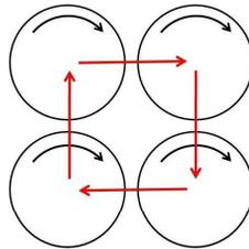
Figure 10: A livelock situation in Mesh of Ring topology
