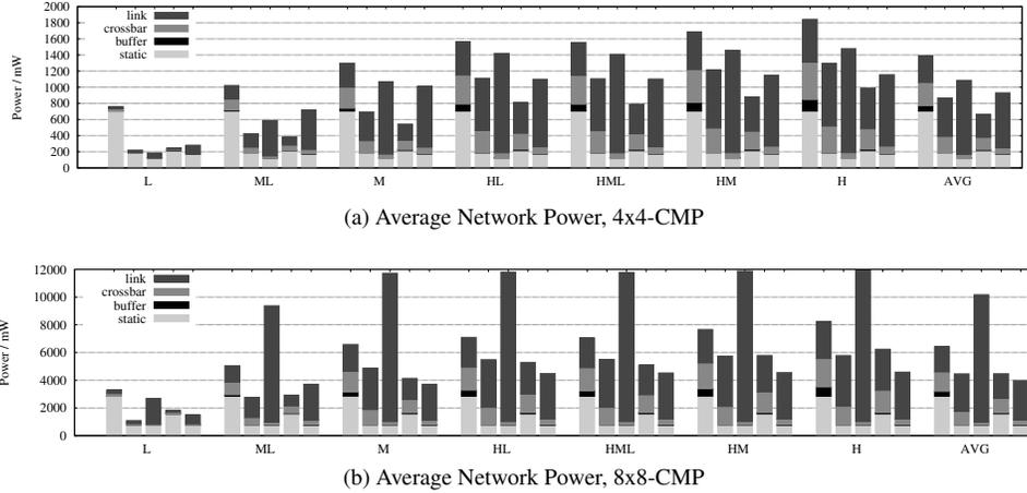
Figure 14: Network power for buffered and bufferless mesh, single and hierarchical ring and mesh of rings networks.(from left to right)
