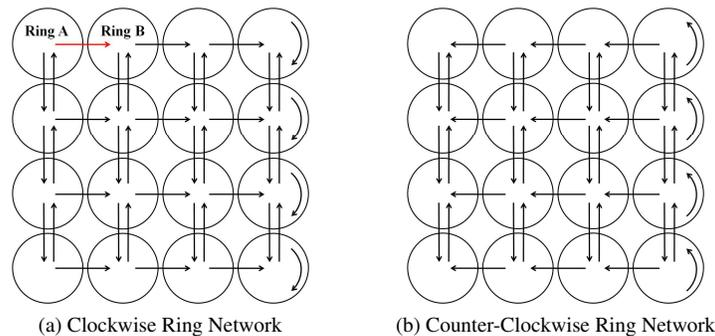
Figure 11: allowed data transfer directions in mesh of rings topology
