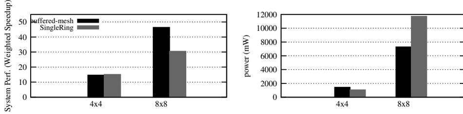
Figure 2: Application performance and average network power as network grows from 16 to 64 nodes in mesh and ring interconnects. Bisection bandwidth is equalized between mesh and ring designs.
