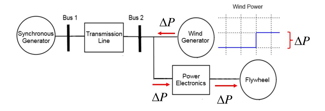
Want to choose set points so that the wind disturbance power goes to the flywheel and rest of the system is minimally affected
