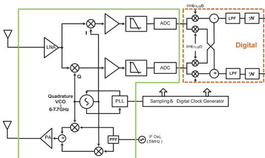
Fig. 1: Transceiver Architecture for SRS system
