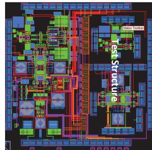
Fig. 2: Layout of SRS Transceiver
